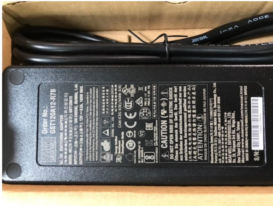
Figure 2-10 AC/DC Power Supply
