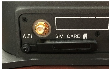
Figure 2-9 Secure the SIM Card Cover
