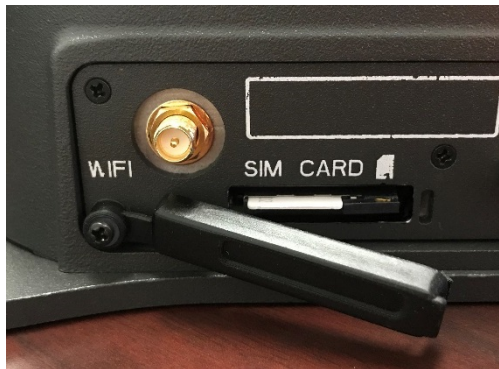
Figure 2-7 SIM Card with Cover Opened
